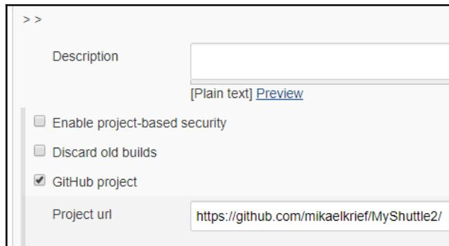
The screenshot shows the 'GitHub project' section of the Jenkins job configuration form. It includes a 'Description' field with a '[Plain text] Preview' link. Below the description are three checkboxes: 'Enable project-based security', 'Discard old builds', and 'GitHub project' (checked). The 'Project url' field contains the URL 'https://github.com/mikaelkrief/MyShuttle2/'.
